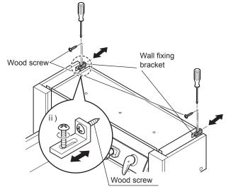
\* If there is gap between the basin body and the wall, fix the basin body on the wall keeping gap.
